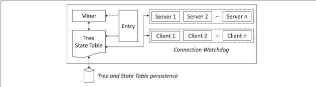
**Fig. 2** Program overview: The mining thread as well as up to *n* server threads and up to *n* client threads operate on the core tree data structure representing the blockchain and the state table representing the assignments of portions. The state of the data structure as well as auxiliary representations like time-slot-accurate portion assignments are persisted to disk. Server and client threads include watchdogs to detect and potentially resume lost connections to other nodes
