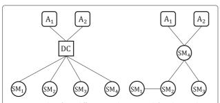
**Fig. 1** Examples of two different topologies (*star, left* and *tree, right*). In the star topology, the data concentrator (DC) collects measurement values from the smart meters (*SM*) and forwards the aggregated values to the aggregators (*A*). In the tree topology measuring values are aggregated in a hop-by-hop manner by the smart meters
