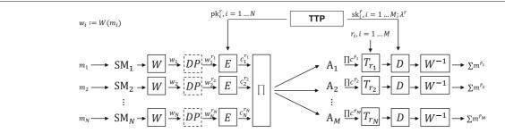
**Fig. 2** MRA aggregation scheme for secure aggregation with homomorphic encryption and multiple aggregators. The component DP representing the addition of Gamma distributed noise is only needed if additionally differential privacy wants to be achieved. In this figure  $w_i := W(m_i)$  denotes the wavelet transform of  $m_i$
