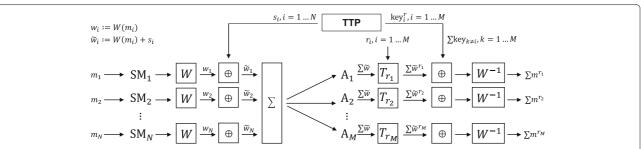
**Fig. 3** MRA aggregation scheme for masking and multiple aggregators. In this figure,  $w_i := W(m_i)$  denotes the wavelet transform of  $m_i$ , and  $\tilde{w}_i := W(m_i) + s_i$  denotes the masked values of  $w_i$
