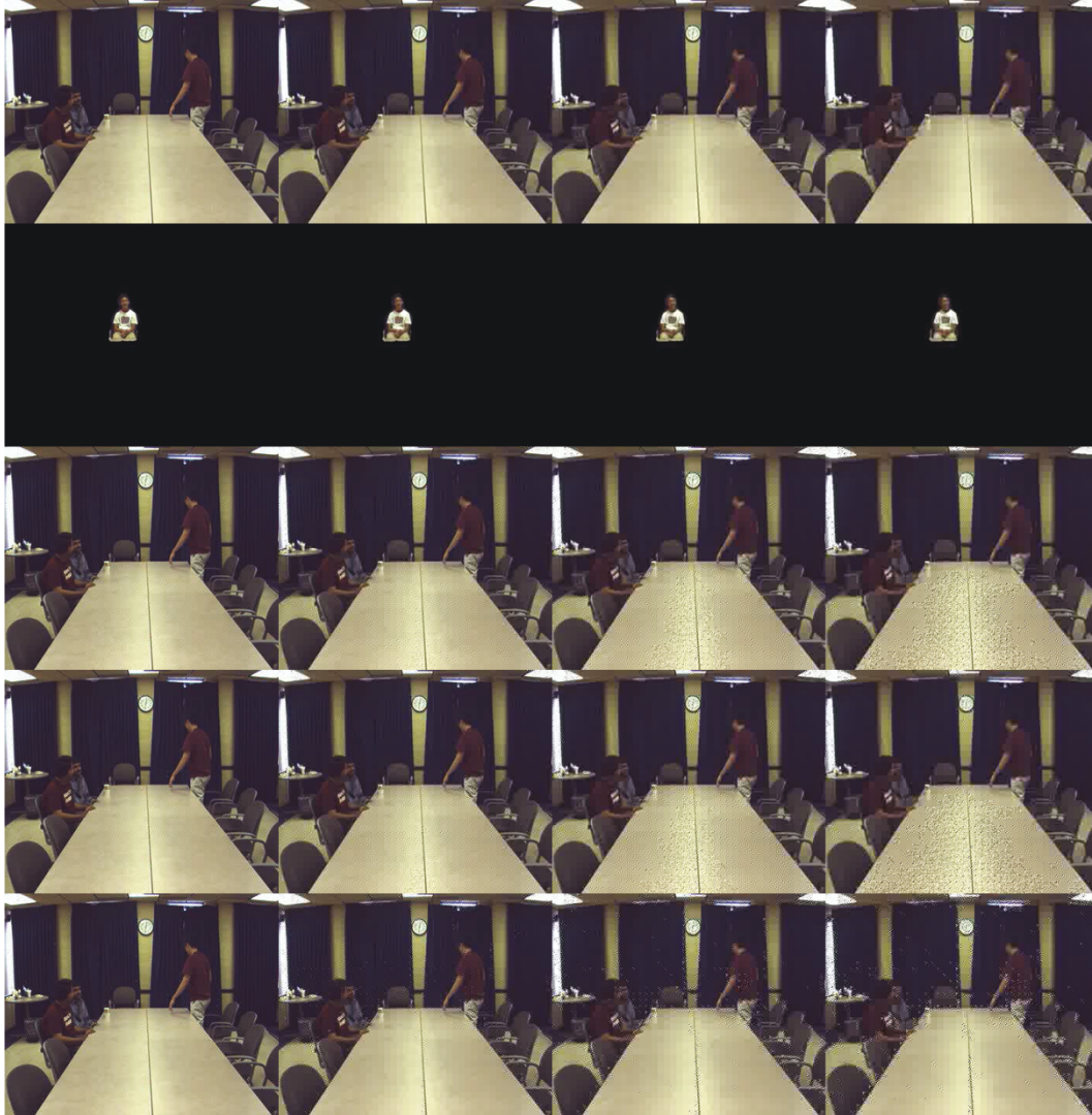
FIGURE 8: Sample frame (200th) from Conference—reversible embedding at varying QP and \delta . Rows from Top to Bottom: Inpainted Frame, Privacy Frame, Data embedded frames with \delta = 0, 0.5 , and 1. Columns from Left to Right: QP = 5, 10, 15, and 20.
