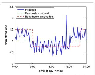
**Fig. 9** Comparison of a worst-case load profile forecast: The load profile forecast (*blue line*) best matches the flat template load profile (*dashed green line*) in the original space, but the night owl profile (*dash-dotted red line*) in the embedded space
