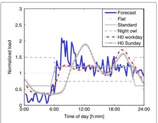
**Fig. 8** Comparison of a load profile forecast and all template load profiles: the H0 workday template load profile (*dash-dotted red line*) matches the forecast (*solid blue line*) best. The inferior matches are depicted in *gray*
