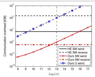
**Fig. 3** Comparison of the communication need of our protocol and the one used for comparison with variable embedding dimension *m*: The communication need for the smart meter is considerably lower with our proposed embedding protocol (denoted *ours*) than with the protocol using homomorphic encryption (denoted *HE*). Utilities only need to send data to the **TP** using our proposed embedding protocol (*blue*, *dashed-dotted*)
