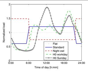
**Fig. 4** Template load profiles: usage-specific load profiles are used as  $\mathbf{L}_{uJ}$  for the *matching* phase
