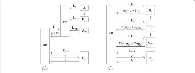
**Fig. 2** Comparison of our proposed scheme (*left*) to approaches using homomorphic encryption (*right*). The latter comes without a third party needed for comparison, which is instead done by the smart meter
