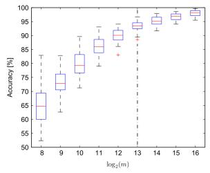
**Fig. 7** Accuracy of the matching process with security parameter  $\Delta=30$  and variable embedding dimension m: The percentage of coinciding best matches based on distance calculations with and without embedding increases with m
