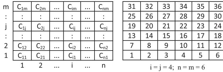
Figure 2 (x, y) coordinate space is divided into cells, and the equivalent cell numbers are shown in right.
