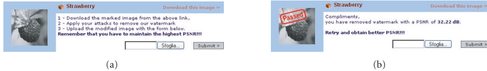
FIGURE 2: The BOWS interface to upload the attacked images and run the detector, as it appears before a successful attack (a), and after a successful attack (b) on the image Strawberry . Note that in case of successful attack the thumbnail of the image shows the stamp “Passed,” and that the PSNR value achieved by the current attack is recorded.
