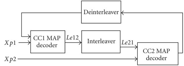
FIGURE 2: Block diagram of the turbo decoder.
