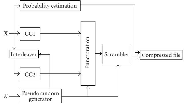
FIGURE 1: Block diagram of the joint encoder.
