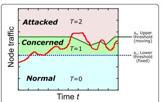
**Fig. 1** Demonstration of dynamic thresholds and the perceived attack state by a node. The *red line* represents the traffic count through the node, as a function of time. The lower threshold  $s_L$  is fixed, but the upper threshold  $s_t$  decreases when traffic exceeds its value, and it increases when traffic is lower than that. In each of the three areas defined by the two thresholds, the perceived threat level of the node assumes the value of either T=0, T=1, or T=2
